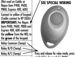
and hold for 3 seconds for PANIC output. Relay can be wired to any zone for an additional panic output.
